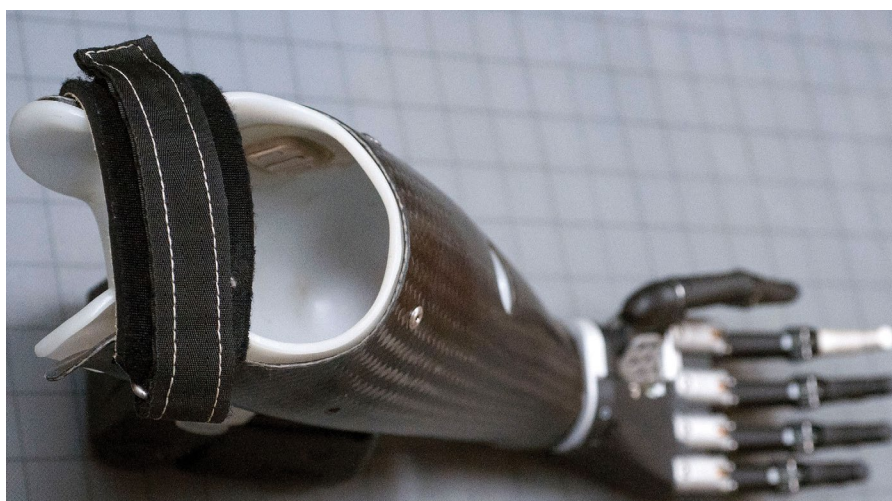
Outer frame of a myoelectric prosthesis and socket
